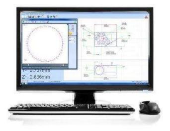
Every time a component is inspected, a programme for measuring subsequent components is automatically created. The software also calculates 'safe' moves between features, even when the probe is indexing – just another thing that the operator doesn't have to worry about!
